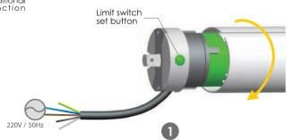
When the brown wire and blue wire connect with 220v/50hz, the drive adapter will rotate in a clockwise direction
