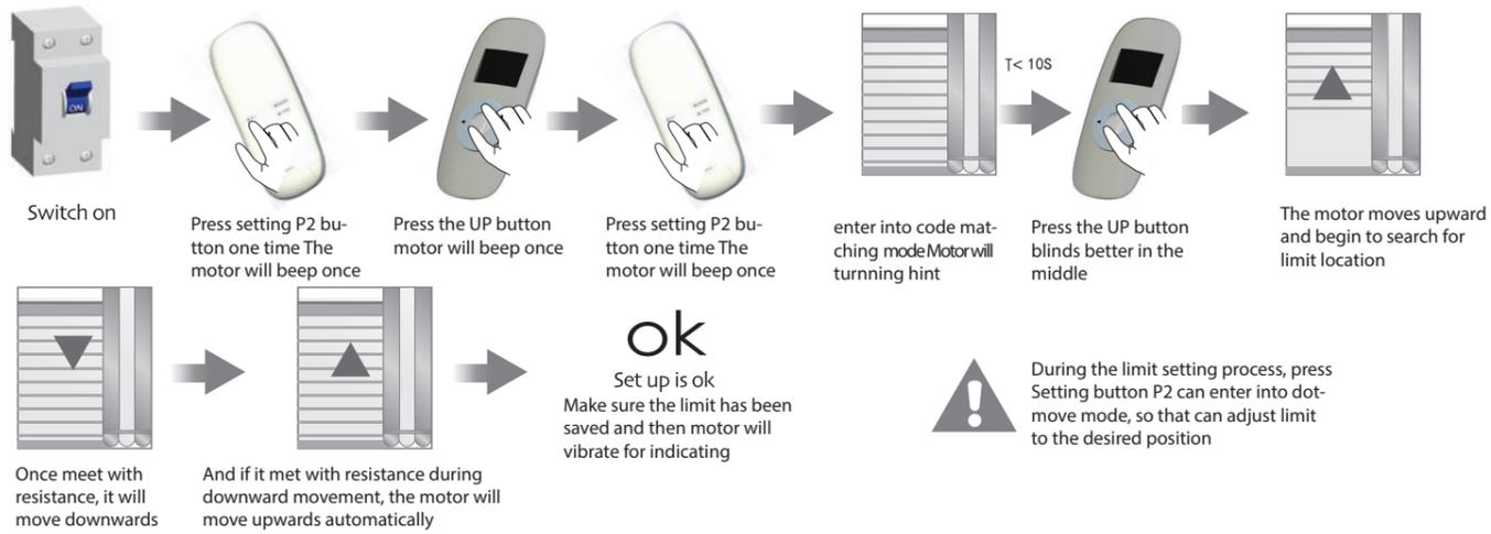
(3) Up and Down limit manual setting should be set before the motor moves upward and meets with resistance when the motor is in Up and Down limit automatic setting mode!
