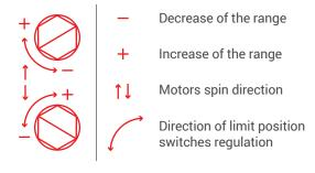
For setting bottom or top limit position roller shutter needs to be started (opening or closing direction) until it stops at the factory set height. For increasing the range of limit position turn the rotary regulator in the '+' direction. Analogically, for decreasing the range, turn in the '-' direction.
