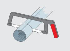
1. Cut the tube to the proper length.
