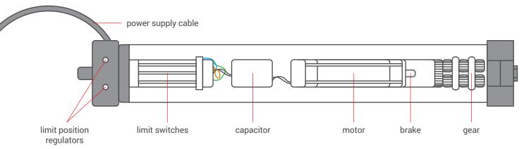
Maximal time of continuous work is 4 minutes. After that time thermal protection will be activated preventing motor form overheating. After that motor will be disabled for about 20 minutes until it cools down.
