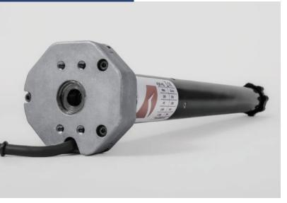
M type motors are designed for automation of roller shutters and garage doors. Motors head is equipped with emergency opening system that allows for gate door or roller shutter to be opened or closed in case of power outage.
