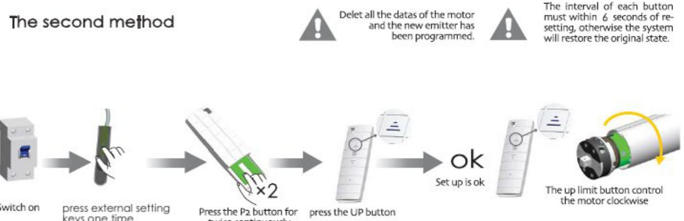
The interval of each button must within 6 seconds of re-setting, otherwise the system will restore the original state.
