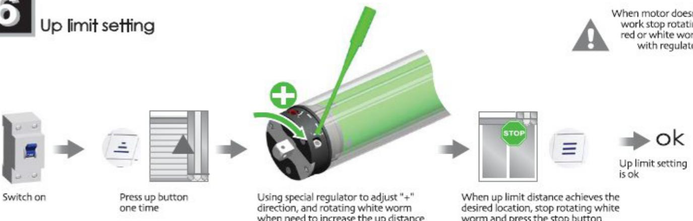
When motor doesn't work stop rotating red or white worm with regulator.
