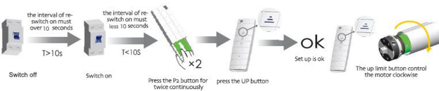
The interval of each button must within 6 seconds of re-setting, otherwise the system will restore the original state.
