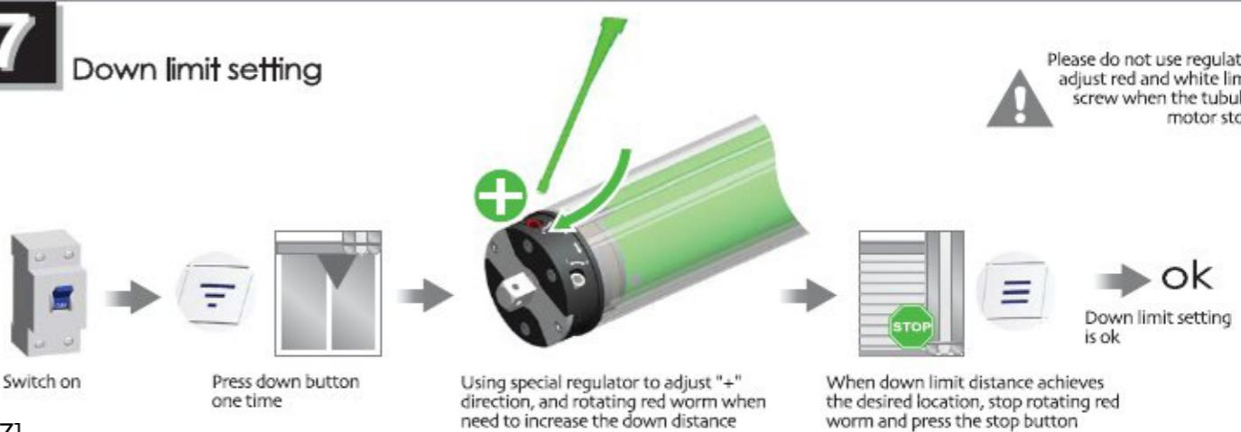
Please do not use regulator adjust red and white limit screw when the tubular motor stop.
