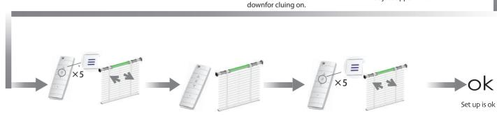
Press the stop button continuously for over 5 times untill the motor roll up and down for hint, that means the upper limit setting successful.
