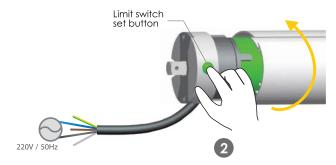
When the drive adapter rotate in a reverse direction or stop(the black wire and blue wire connect with 220v/50hz), press the setting button in the limit head, the motors will rotate in a reverse direction
