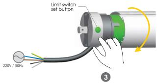
Release the setting button in the limit head namely confirm clockwise limit position
