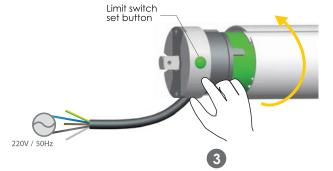
Release the setting button in the limit head namely confirm reverse limit position
