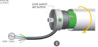
When the brown wire and blue wire connect with 220v/50hz, the drive adapter will rotate in a clockwise direction
