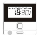
Press "Time set button" , the down timing time (minute mark) of this channel twinkles
