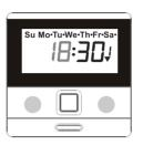
Press "up button" or "down button" to adjust the down timing time (hour mark) of display screen.
