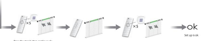
Press the stop button continuously for over 5 times untill the motor roll up and down for hint, that means the upper limit setting successful.
