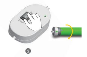
Press the UP button in the DC270, the motors will rotate in a clockwise direction or stop
