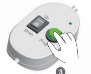
Press the Program button in the DC270, the motors will rotate in a Counter-clockwise direction, Release the Program button namely confirm Counter-clockwise limit position
