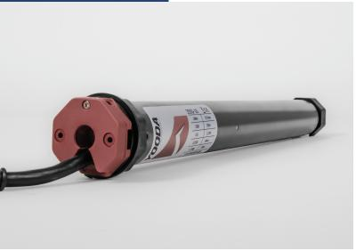
S type motors are designed for automation of roller shutters blinds and shutters or roller garage doors. They can also be controlled by a wall switch or throughout additional radio receiver. Motors are equipped with mechanically set limit positions allowing roller shutter to stop on desired level.
