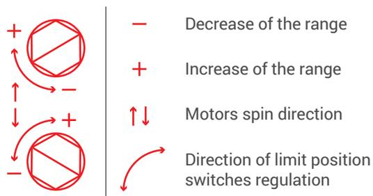
For setting bottom or top limit position roller shutter needs to be started (opening or closing direction) until it stops at the factory set height. For increasing the range of limit position turn the rotary regulator in the '+' direction. Analogically, for decreasing the range, turn in the '-' direction.
