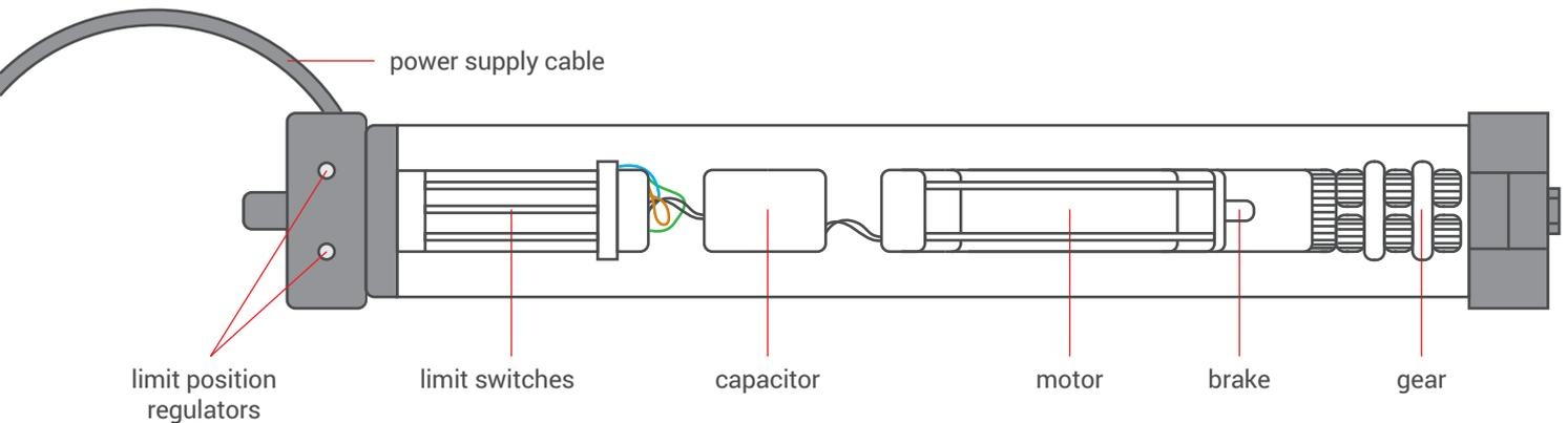
Maximal time of continuous work is 4 minutes. After that time thermal protection will be activated preventing motor from overheating. After that motor will be disabled for about 20 minutes until it cools down.
