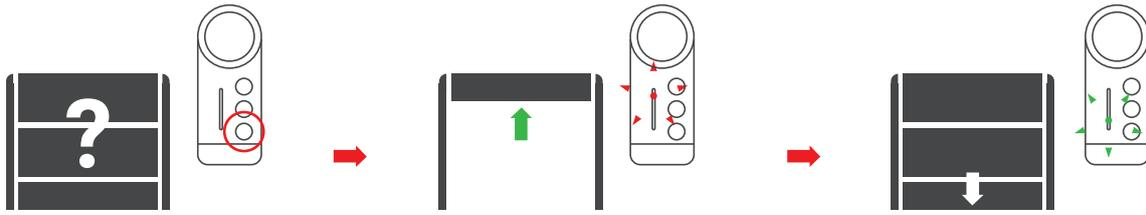
To check the garage door's position, press the status button on the transmitter, then press the button which controls the garage drive.
