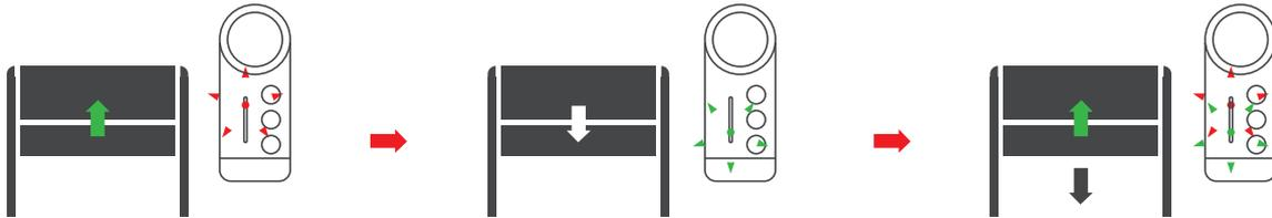
When the red LED diode flashes, the door is opening.
