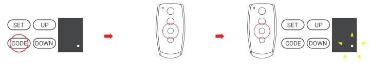
Press CODE button. In the bottom corner a dot (.) appears. Press the button on the transmitter that will control the drive.
