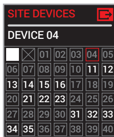
Switching between channel numbers is performed by pushing UP, DOWN, CHANNEL+ or CHANNEL- buttons or by using joystick. Activating and deactivating highlighted channel can be done by pushing STOP button or joystick.
