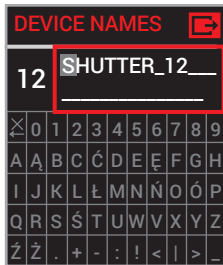
Using UP, DOWN, CHANNEL+, CHANNEL- buttons or joystick switch to sign you want to change (sing is flashing). Confirm the change by pushing STOP button or joystick.
