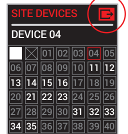
When exit button is highlighted pushing STOP button or joystick will make remote return to MENU screen.
