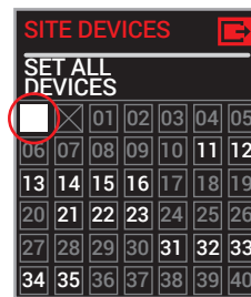
By choosing white square all channels are activated. By choosing all channels are deactivated.
