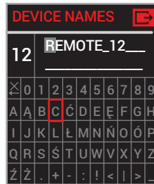
Using UP, DOWN, CHANNEL+, CHANNEL- buttons or joystick select the sign to which you want to change already previous sign (sing is flashing). To confirm the change press STOP button or joystick. That step automatically switches name editing to the next sign.
