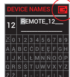
When exit button is highlighted pushing STOP button or joystick will make remote to return to MENU screen.
